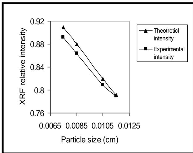
Figure 6: XRF relative intensity as a function of particle size for Ni powders suspended in Iraqi oil
