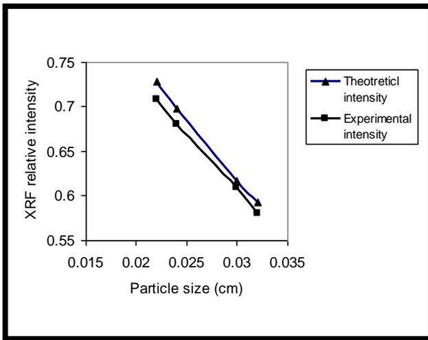
Figure 4: XRF relative intensity as a function of particle size for Fe powders suspended in Iraqi oil
