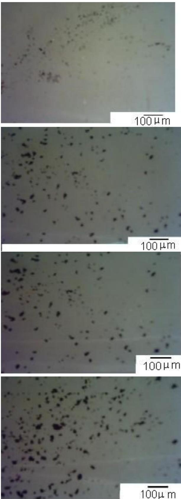
Figure 2: Microscopic photograph of Cobalt nanoparticles suspended in oil at different particle sizes .x100
