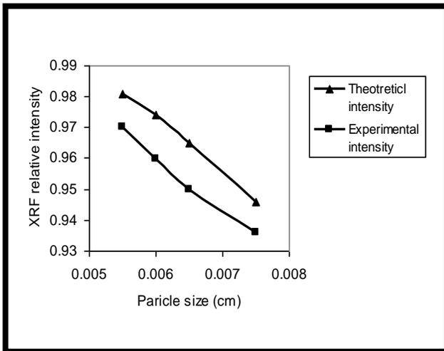
Figure 5: XRF relative intensity as a function of particle size for Co powders suspended in Iraqi oil.
