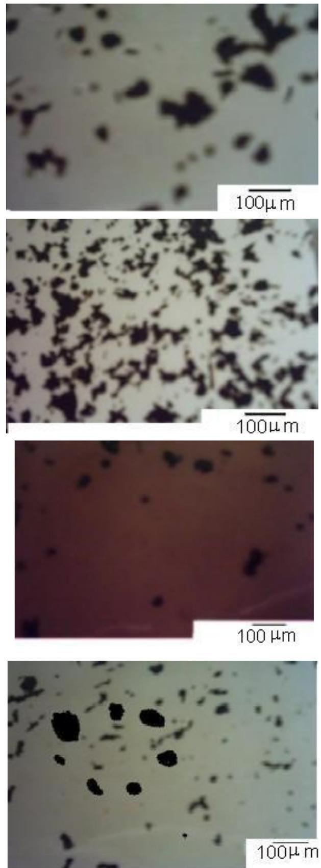
Figure 3: Microscopic photograph of Nickel powder suspended in oil at different particle sizes x100
