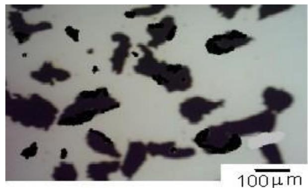
Figure 1: Microscopic photograph of Iron nanopowder suspended in oil at different particle sizes x 100
